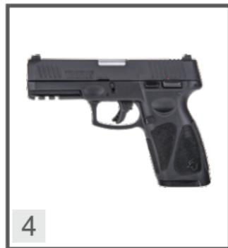
After the last round, remove the magazine, the slide will remain in the open position held by the slide catch. In order to make it return to its rest position, press the slide catch downward just above the left grip or pull slide to the rear and let same go forward.
