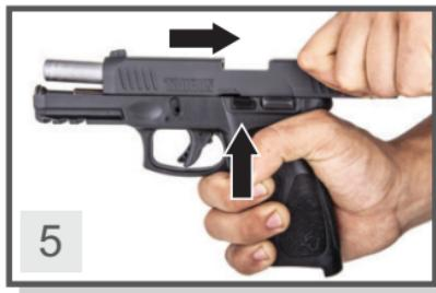
If you want to stop shooting before firing the last cartridge of a magazine, push the safety lever (when available) in the up (on) position.
